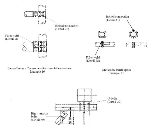
Beam-Column Connection for Truss Structure Example 18
